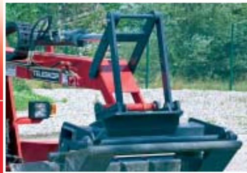
Standardized quick tool-change frame, Euro Standard
