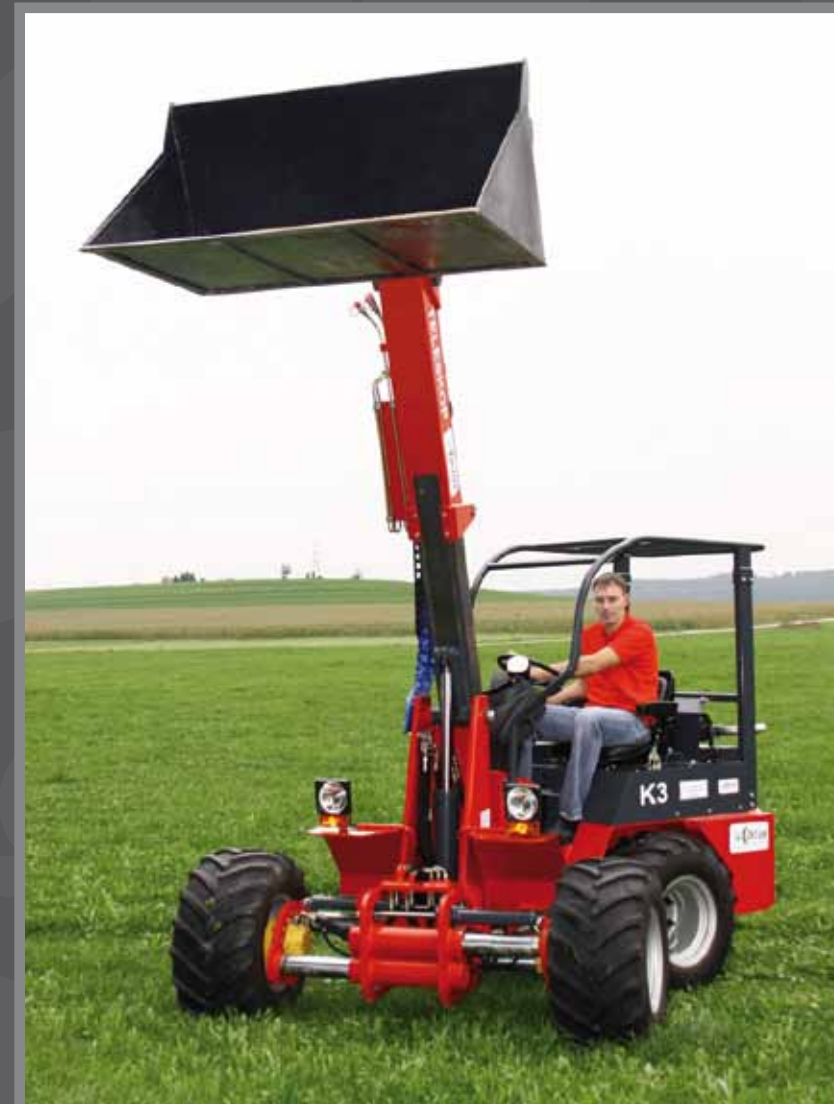
Thanks to the tool holding fixture, which meets the DGS Euro standard, commercially available tools can be used.
